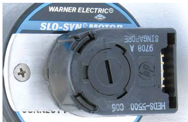
Rotary encoder mounted to motor shaft extension
