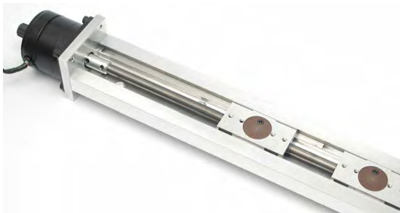
Example 4: UniSlide Assembly with two sliding carriages and a left and right hand threaded lead screw for simultaneous reciprocal motion. This design is useful for alignment and centering operations.
